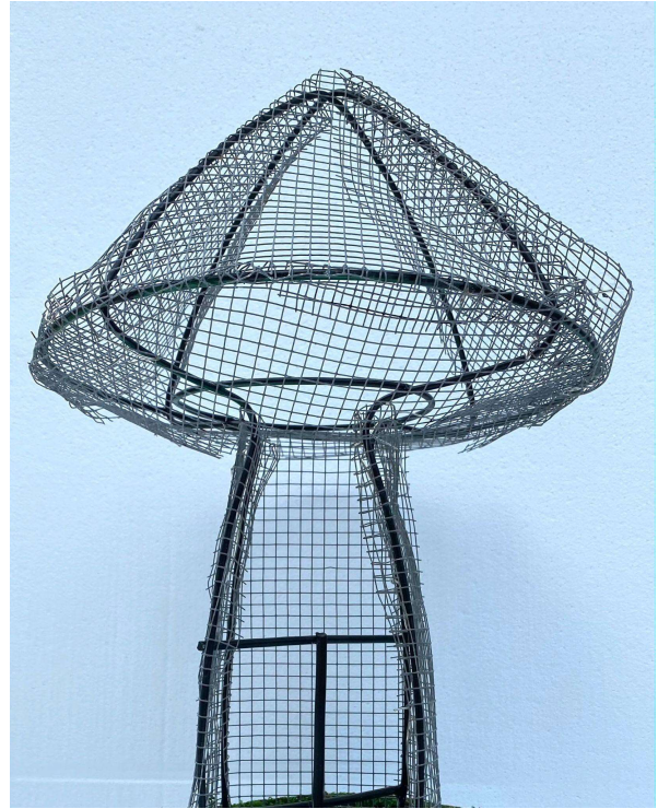
2. Steel mesh wired to frame in preparation for fiberglass cloth to be coated with resin as seen in next photo
