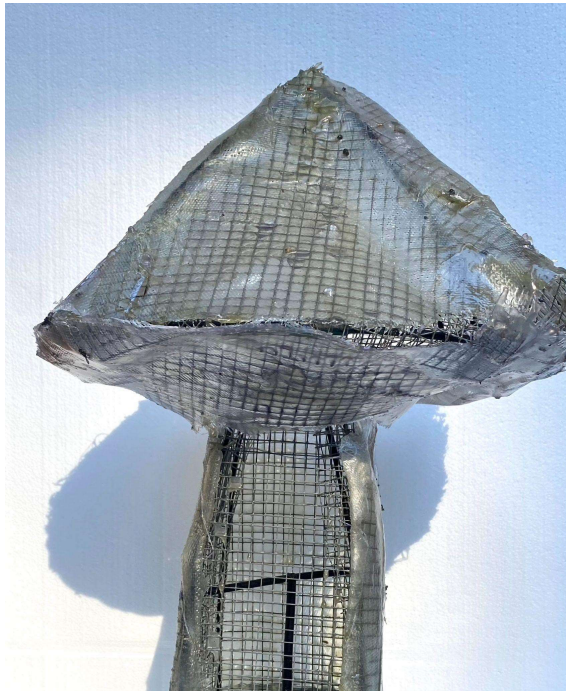
3. Fiberglass and resin hardened over the form
